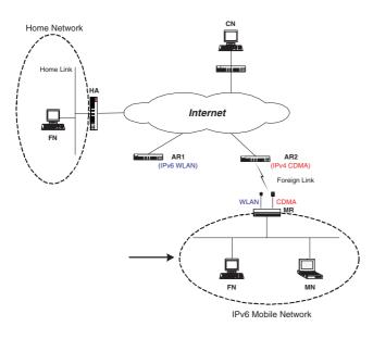
Fig. 2. IPv6 Mobile Network moving into IPv4 Access Network
