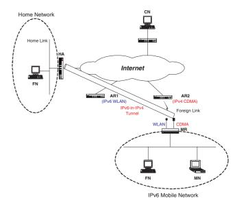
Fig. 3. Setup of IPv6-in-IPv4 Tunnel
