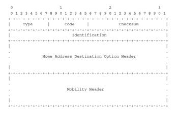
Fig. 6. Dynamic Tunnel Management Protocol (DTMP) Message Format
