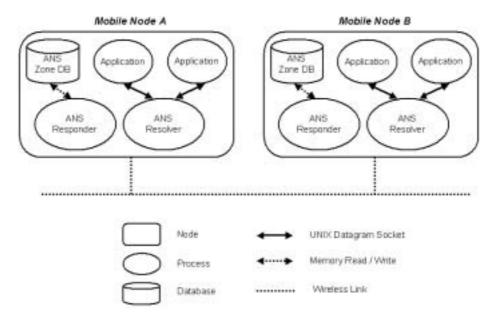
Fig. 2. ANS System for Name Service in IPv6 MANET
