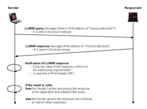
Fig. 1. Procedure of the Resolution from Domain Name to IPv6 Address in LLMNR
