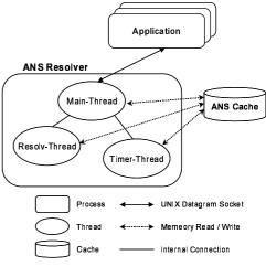
Fig. 3. Architecture of ANS Resolver
