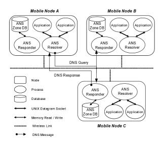
Fig. 1. DNS Name Resolution through Ad Hoc Name Service System (ANS)
