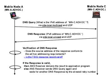
Fig. 5. Procedure of Secure DNS Resolution through TSIG Resource Record
