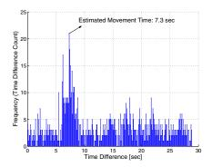
Fig. 5. Estimation of Movement Time through TDOD Operation
