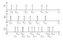
Fig. 3. Detection Sequence for Vehicles at Sensors  $s_1$ ,  $s_3$ , and  $s_2$
