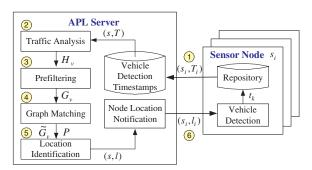
Fig. 2. APL System Architecture
