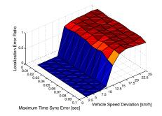
Fig. 13. APL Operational Region for Maximum Time Synchronization Error and Vehicle Speed Deviation
