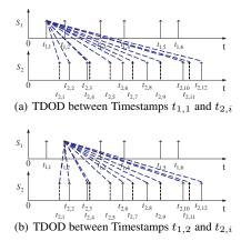
Fig. 4. Time Difference On Detection for Sensors  $s_1$  and  $s_2$
