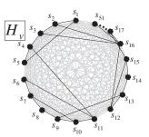
(b) Virtual Topology of Wireless Sensors:  $H_v = (V_v, M_v)$
