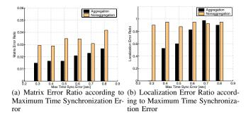
Fig. 9. Performance Comparison between Aggregation and Nonaggregation Methods for Maximum Time Synchronization Error  $(\epsilon_{max})$
