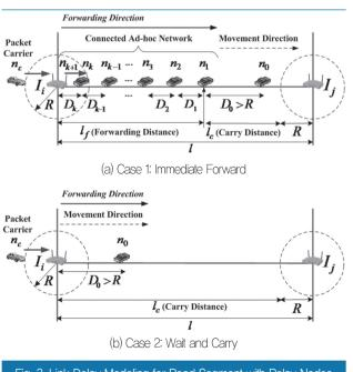
III.1.2 Link Delay for Road Segment with Relay Nodes
