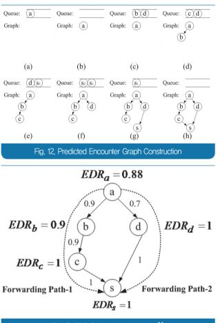
Fig. 13. EDR Calculation of Vehicle  $V_a$
