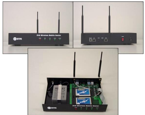
Fig. 6. IPv6 Wireless Mobile Router
