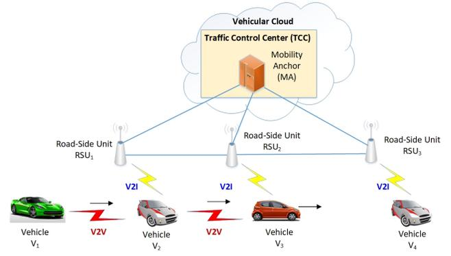
Fig. 1. Vehicular Network Architecture
