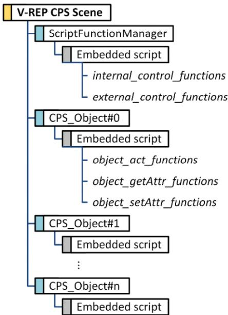
**Figure 2: Structure of V-REP Simulation**
