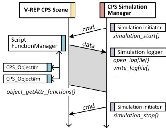
Figure 4: Sequential Diagram of Simulation Manager
