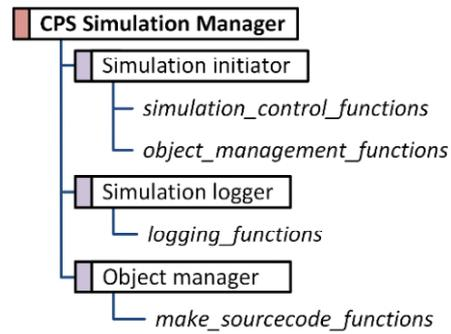
**Figure 3: Structure of Simulation Manager**
