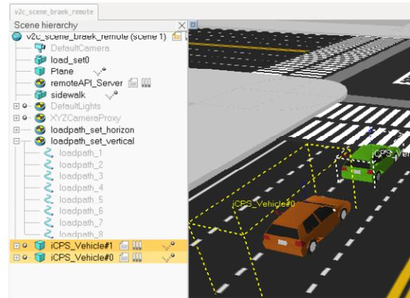
Figure 6: V-REP Simulation of Intelligent Transportation Systems
