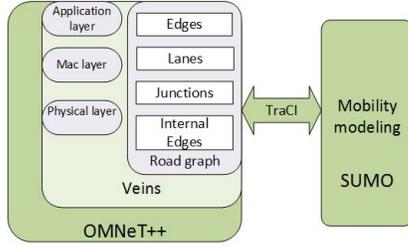
Fig. 1. OMNeT++ and SUMO communicate through TraCI in Veins
