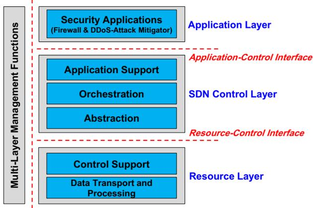
Fig. 2. High-level Architecture for SDN-based Security Services
